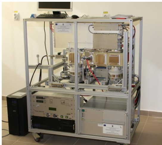
Spectrometru de masa AMS Aerodayne
