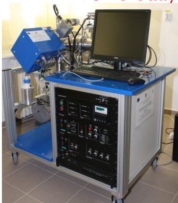
Spectrometru de masa AMS Aerodayne
