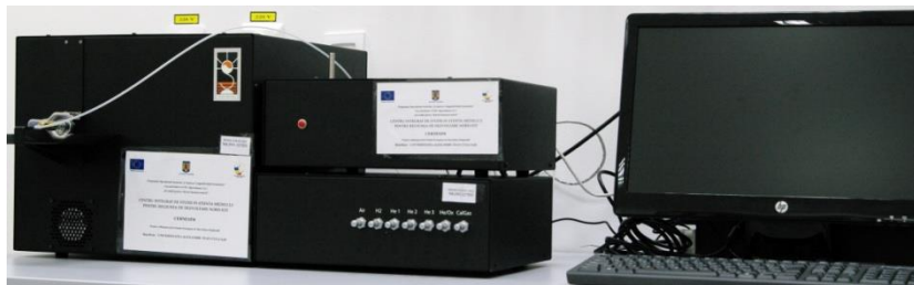
Analizor OC/EC SUNSET Laboratory Inc.
