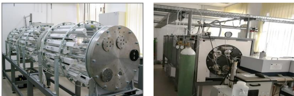
Figure I.17. The ESC-Q-UAIC reaction chamber and the chamber's inlet flange.
