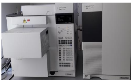
Figure II.2 Agilent 7890A GC / Agilent 240 Ion Trap GC/MS gas chromatograph and the main components of the instrument ( Agilent 240 Ion Trap GC/MS, 2011 )
