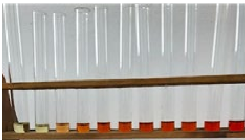
Figure II.5.6. Pauly reaction of histidine (concentrations 0–300 µg/mL) with diazotized sulfanilic acid.
