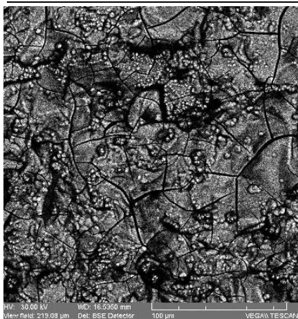
Figure 1. Co-deposition of zinc-nickel alloy on gold plated glass, at -1000 mV, 2 hours and 30°C (optical increase factor 1000×).
