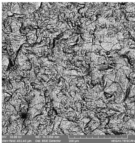
Figure 5. Co-deposition of zinc-nickel alloy on gold plated glass, at -1050 mV, 2 hours and 30°C (optical increase factor 1000×)
