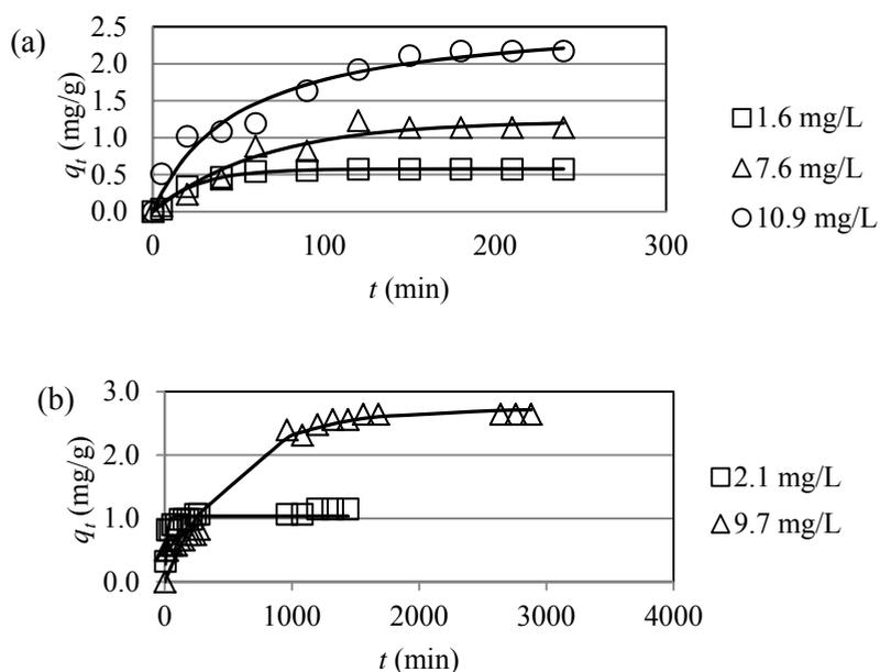
**Figure 2.** Rate of (a) Methylene Blue, and (b) Reactive Orange 16 adsorption onto carbon-based beta-cyclodextrin adsorbent (lines were predicted by pseudo-first-order model).
