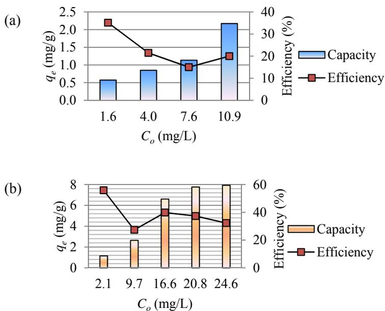
**Figure 3.** Performance of carbon-based beta-cyclodextrin adsorbent for (a) Methylene Blue and (b) Reactive Orange 16 removal.
