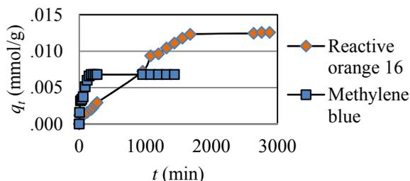
**Figure 4.** Rate of dyes adsorption at the same molar concentration of 0.034 mM by carbon-based beta-cyclodextrin adsorbent.
