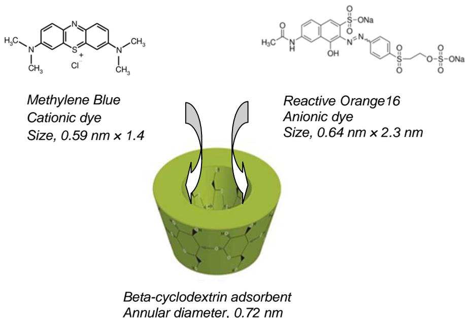
**Figure 5.** Illustration of dyes adsorption onto carbon-based  $\beta$ -CD.
