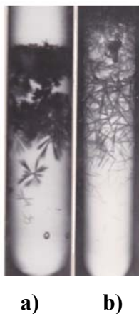
Figure 3. Interchanging the reactant: (a) 0.2 N oxalic acid above gel and 0.5 N BaCl 2 inside gel; (b) 0.2 N BaCl 2 above gel and 0.5 N oxalic acid inside gel.
