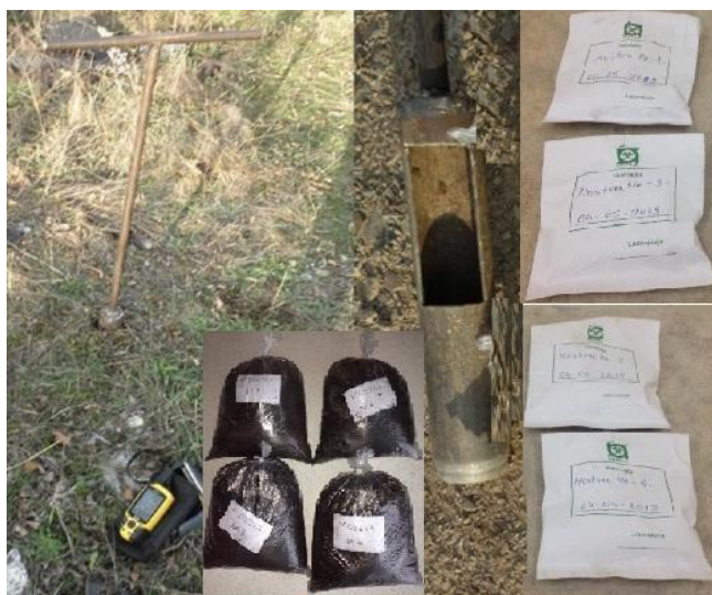
Figure 6. Obtaining soil samples by means of a metal probe and marking them.
