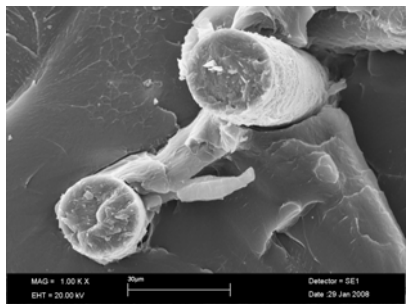
Figure 12. Fractured surface of fiber + HEA group under SEM (X 1000 magnification).
