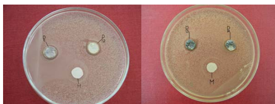
Figure 1. Antibacterial test results using Escherichia coli ATCC 25922 (P 1 -P b treated with AgNO 3 , P 2 -P a treated with AgNO 3 , P 3 -P b ion exchange with Ag + and reduced with CH 2 O and P 4 -P a ion exchange with Ag + and reduced with CH 2 O, M – blank sample)
