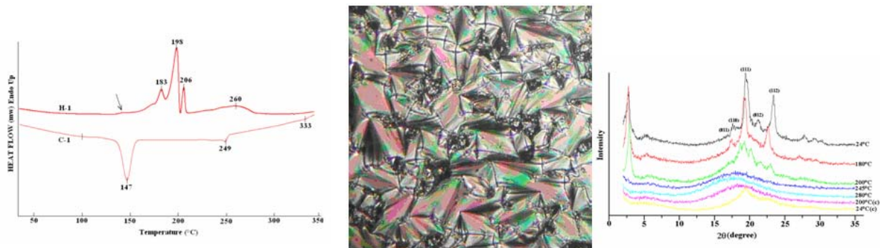
Figure 1. DSC curves, optical micrograph and XRD pattern at different temperatures of synthesized polymers.
