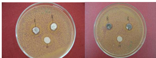
Figure 2. Antibacterial test results using Staphylococcus aureus ATCC 25923 (P 1 -P b treated with AgNO 3 , P 2 -P a treated with AgNO 3 , P 3 -P b ion exchange with Ag + and reduced with CH 2 O și P 4 -P a ion exchange with Ag + and reduced with CH 2 O, M – blank sample)
